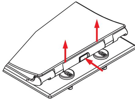
(4) The toilet cover is kept in a graphic orientation, and the button is pressed, and the toilet cover is pulled out from the hinge base.
