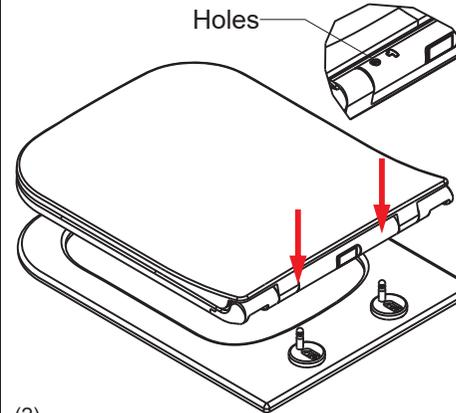
(2) Keeping seat and cover in the icon position, insert the holes of seat and cover into the hinge.
