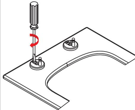
(5) Fully tighten the screws.
